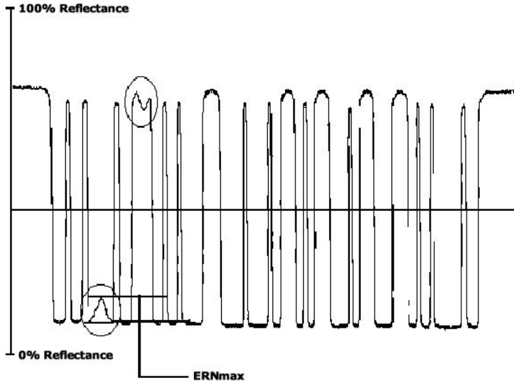
Figure 14 - Grade 4/A Defects
