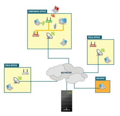
Figure 2: Overview of the AirDefense Wireless Intrusion Detection and Prevention System for wireless security policy enforcement.
