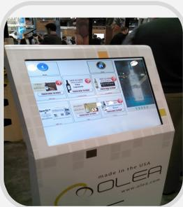
There is a convergence of several technologies that needed to come together to make this offering a success. This solution includes a touch screen computer enabled with Touch Coupon Software, a Zebra Technologies KR203 kiosk printer, and an M2M modem for real-time communication with each of the remote locations.
